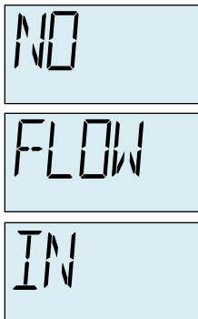
Figure 3-4 NO FLOW IN Alarm
