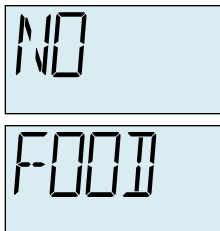
Figure 3-6 NO FOOD Alarm
