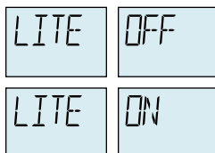
Figure 2-29 Backlight Settings LITE OFF and LITE ON
