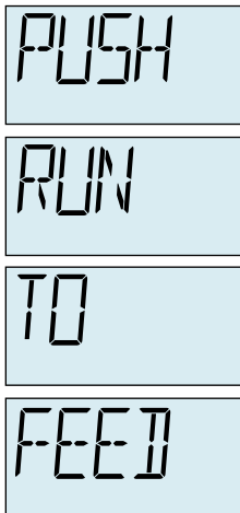
Figure 3-7 PUSH RUN TO FEED Alarm
